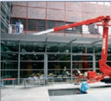
Due to articulated telescopic boom construction many obstacles can be overcome
