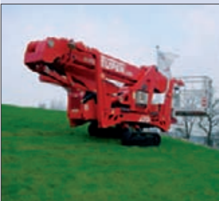
Adjustable crawler chassis permits driving on slopes
