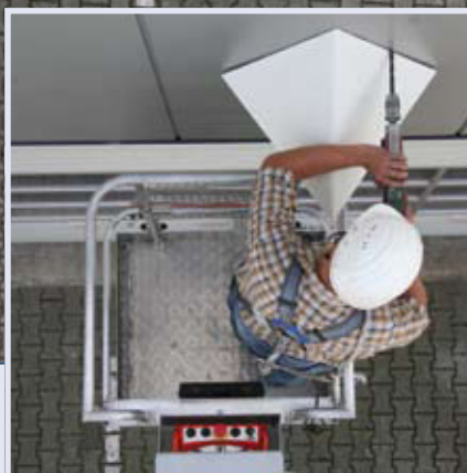
The new basket design allows two persons to work directly at building site. As additional advantage, it can quickly be changed to a one-man basket.
