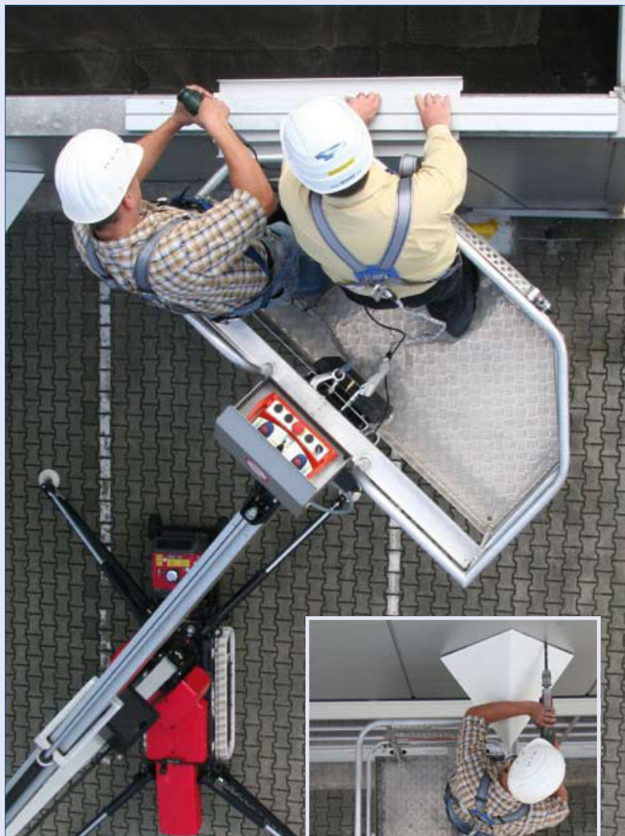
The new basket design allows two persons to work directly at building site. As additional advantage, it can quickly be changed to a one-man basket.
