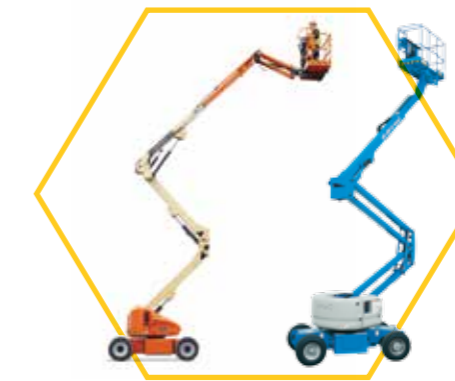
Electric Articulated Booms Working height from 14.19m – 20.39m
