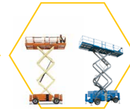
Diesel Scissor Lifts Working height from 9.92m – 34m
